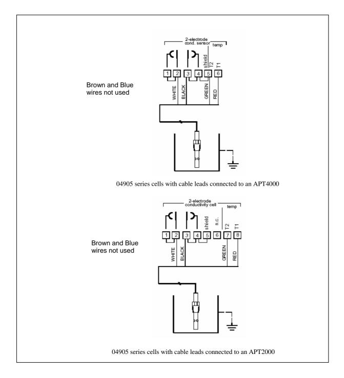
Figure 4-3 4909/4908 Series to APT Series Analyzer/Transformer
