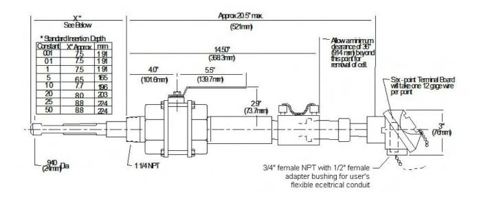
Figure 3-4 Outline and Dimension Drawing for Insertion/Removal Mounting and Cell with Junction Box Head
