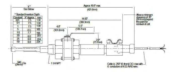
Figure 3-5 Outline and Dimension Drawing for Insertion/Removal Mounting and Cell with Cable
