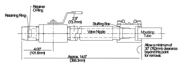
Figure 3-3 Cell Assembly Dimensions and Parts Identification
