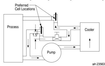
Figure 3-1 Recommended Locations for Mounting a Conductivity Cell
