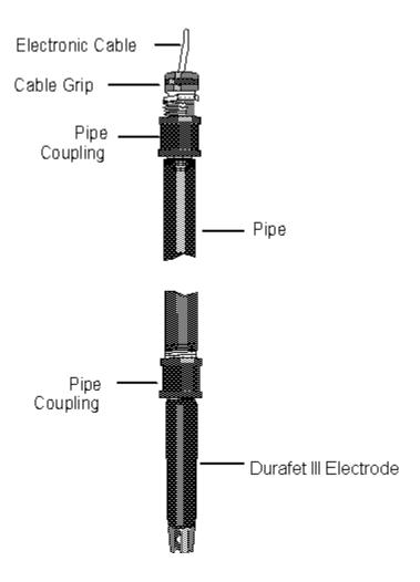
Figure 8-2 Direct Electrode-to-Instrument Connection
