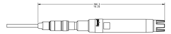
Figure 3-4 Durafet III (Vario Pin Connector) pH Electrode for Immersion Mountings (Guarded Tip), with cable
