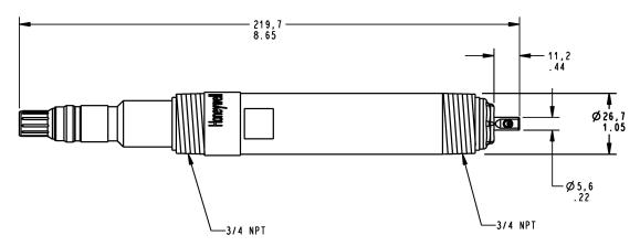
Figure 3-1 Durafet III (Vario Pin Connector) pH Electrode for In-Line Mountings (Smooth Tip)
