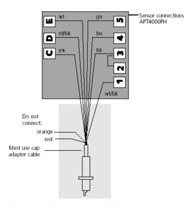
Figure 7-3 Connecting to an APT4000 pH Analyzer
