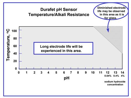
Figure 1-1 Temperature vs. Alkali Resistance
