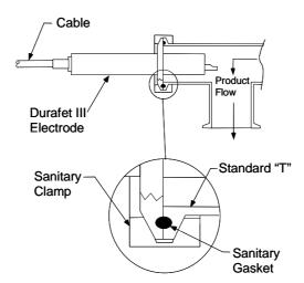
Figure 2-2 Electrode Installation in Tee
