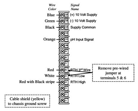
Figure 2-5 Terminal Designations for Durafet III Electrode with Cap Adapter
