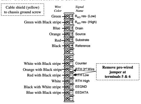
Figure 2-4 Terminal Designations for Durafet III Electrode
