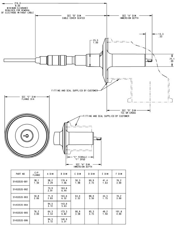
Figure 2-1 Sanitary Durafet III Electrode Outline and Dimensions
