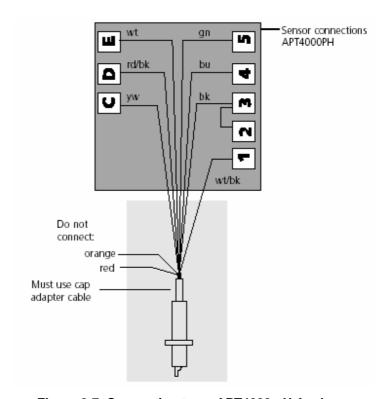
Figure 2-7 Connecting to an APT4000 pH Analyzer
