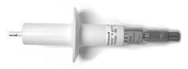
The Sanitary Durafet III pH electrode has an integral, tri-clamp flange for easy mounting in the process. Cable options are available for remote mounting to the innovative UDA2182 Dual Input Analyzer. It is also available with the Cap Adapter cable for connection to Honeywell instrumentation (APT and UDA2182 Series), as well as selected competitors' instrumentation. All cable options use the Vario Pin connector that provides an IP68, waterproof connection to the electrode.
