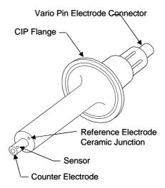
Figure 1-1 Sanitary Durafet III pH Electrode
